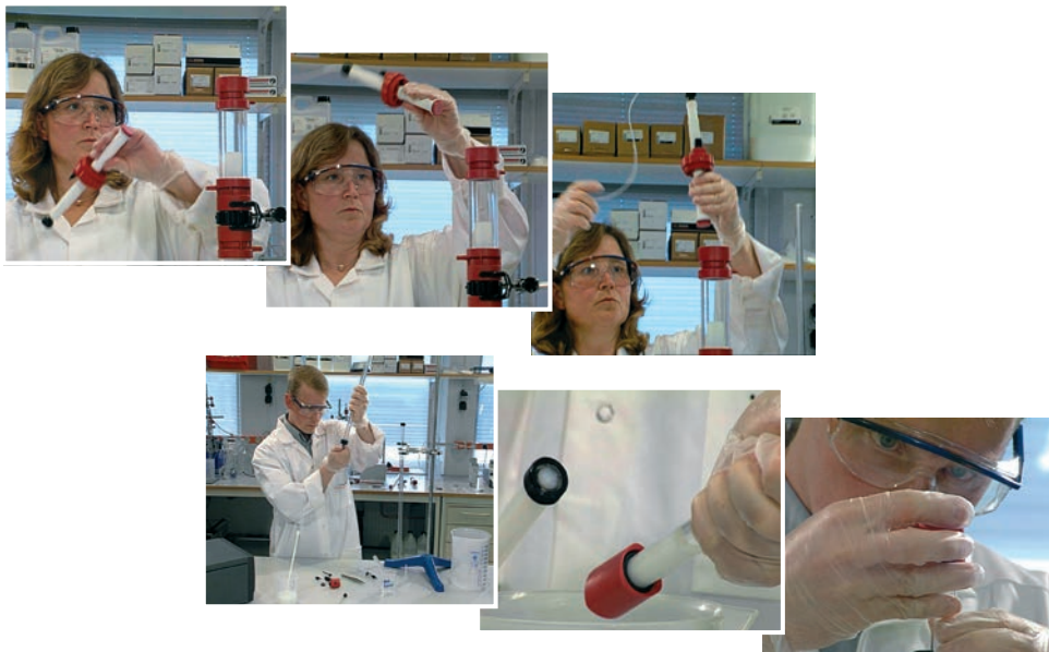
Fig A6.1. Column packing in progress.
