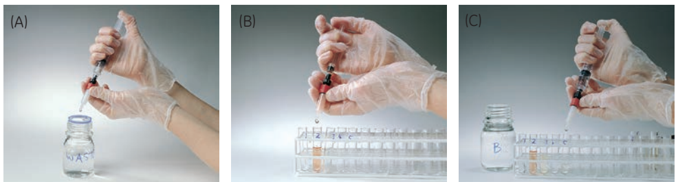
Fig 5.9. Using a GSTrap column with a syringe. A) Prepare buffers and sample. Remove the column's top cap and snap off the end. B) Load the sample and begin collecting fractions. C) Wash and elute, continuing to collect fractions.
